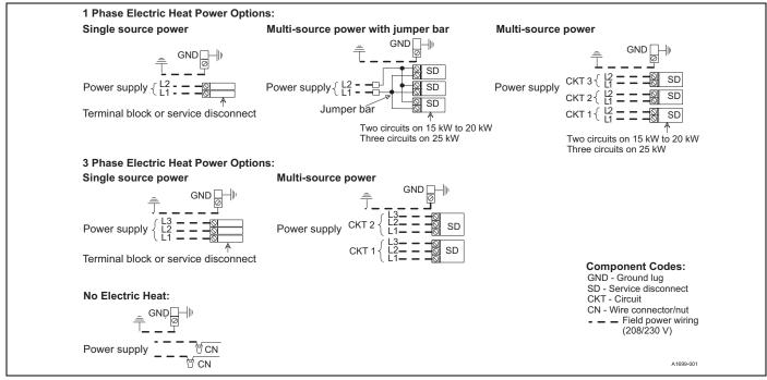
Figure 10: Line power connections
