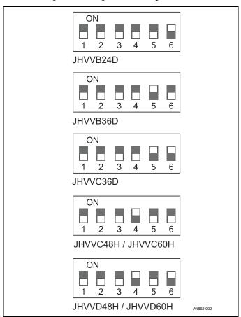
Figure 15: DIP switch settings by model
