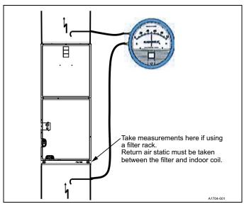
Figure 19: Duct static measurements
