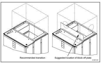
Figure 8: Ductwork transition
