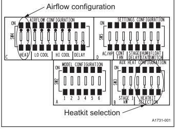
Figure 18: Variable speed board dip switch locations - heat kit
